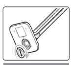
Re-insert the **Attachment Nut** into the bottom of the **Light Stand** and tighten.
